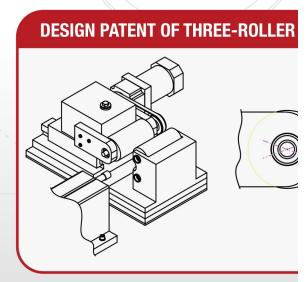
No matter what the diameter of the w putting on the fixture, the center of the the same line and the concentricity w the same workpiece is repeated pick
